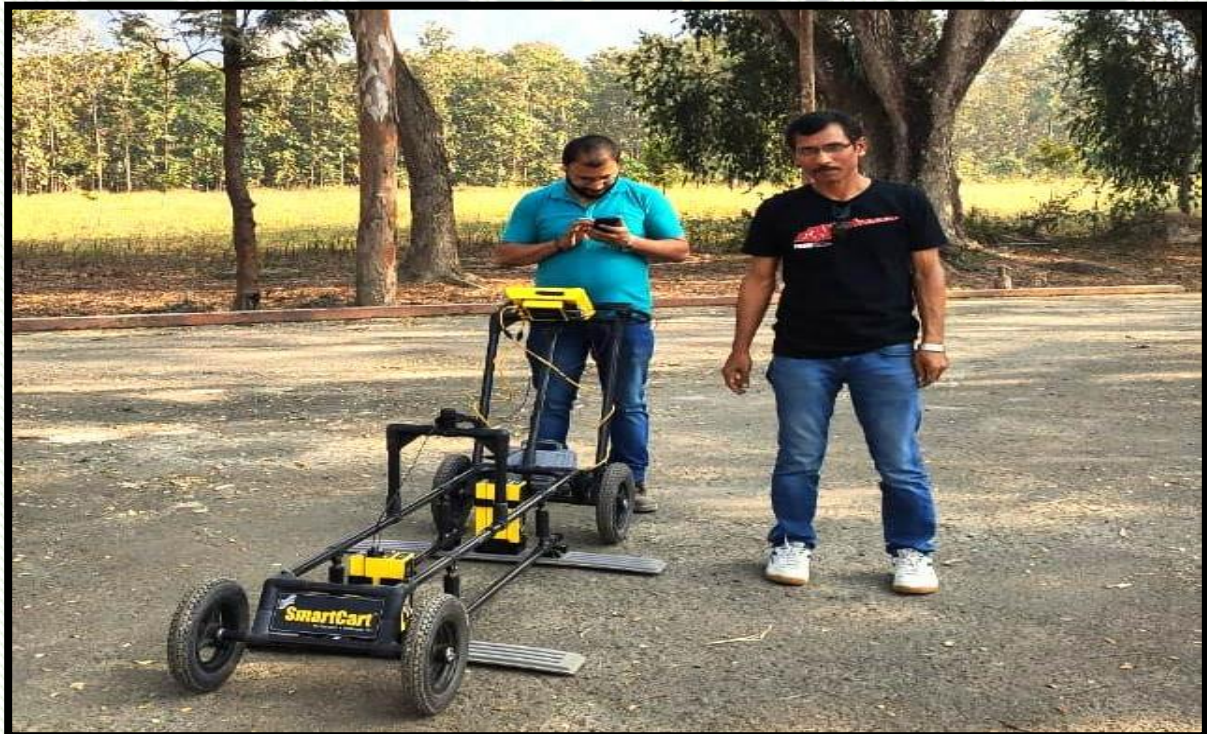
Dr. Manoj K. Phukan, Senior Scientist and Mr. Sausthov M. Bhattacharyya, Technical Officer of GSTD, CSIR-NEIST conducting Geophysical survey using GPR (Ground Penetrating Radar) at CSIR-NEIST premises for detection of underlying water pipes, cables etc.
