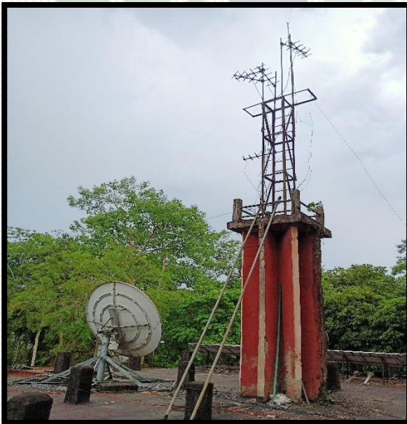
Digital Seismic Telemetry System comprising digital telemetry remote stations located at 27 different sites of North East India and an on-line event detection and data recording station at CSIR-NEIST Jorhat [operated during 1990 - 1998]
