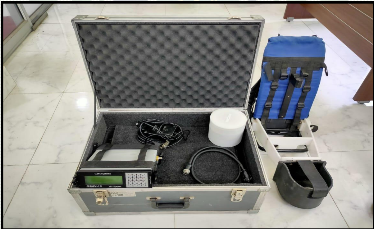
Highly versatile Very Low Frequency (VLF) Electromagnetic System of GSTD. VLF is a geophysical ground probing technology that utilizes VLF signals in the 15 to 30 kHz range normally used for communication with submarines. The signal generated is suitable for making geophysical measurements globally.
