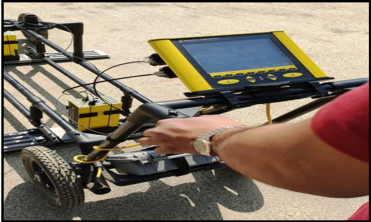
A Ground Penetrating Radar (GPR) of GSTD. Ground-penetrating radar is a geophysical method that uses radar pulses to image the subsurface. It is a non-intrusive method of surveying the sub-surface to investigate underground utilities such as concrete, asphalt, metals, pipes, cables or masonry.
