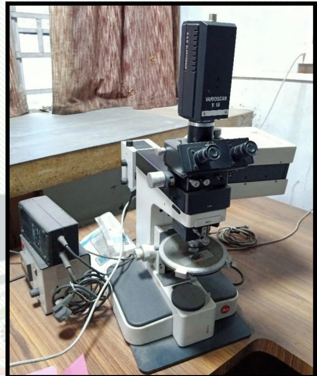
Petrographic microscope facility at GSTD, CSIR-NEIST for mineralogy studies: Stereo Microscope & Leit3 Microvid Microscope. A petrographic microscope is a type of optical microscope used in petrology and optical mineralogy to identify rocks and minerals in thin sections.
