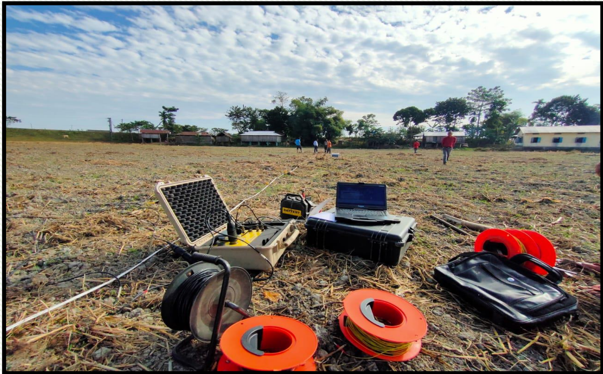
A Multichannel analysis of surface waves (MASW) system with 48 Channel Seismographs. MASW is a seismic exploration method for determination of near-surface shear wave velocity profiles based on analysis of horizontally travelling Rayleigh waves.
