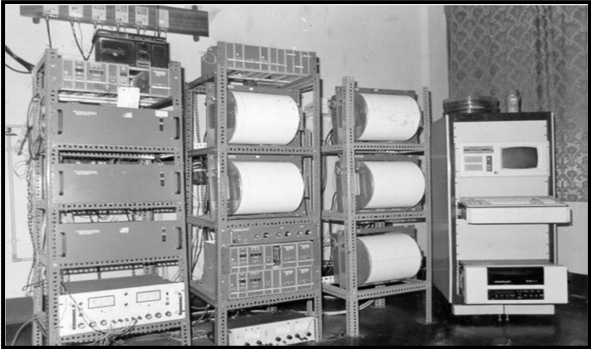
Digital Seismic Telemetry System comprising digital telemetry remote stations located at 27 different sites of North East India and an on-line event detection and data recording station at CSIR-NEIST Jorhat [operated during 1990 - 1998]
